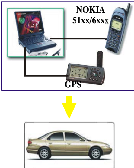
Fig. 5. The block scheme of the measuring system for measuring the signal level of the active GSM system.
