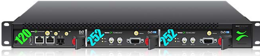
Figure - The 1RU Enhanced Chassis populated with one VB120 module controlling two VB252 DVB-T/T2 input modules giving a total of 4 independent RF inputs.
